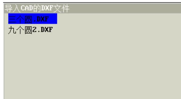
the SD card, press the "OK button", you can start to convert the graphics file to the project file used by this system.
