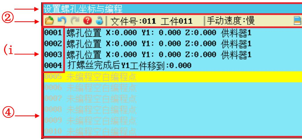
⑤ Figure 0 .1 The "Setting the screw hole coordinates and programming" window.
