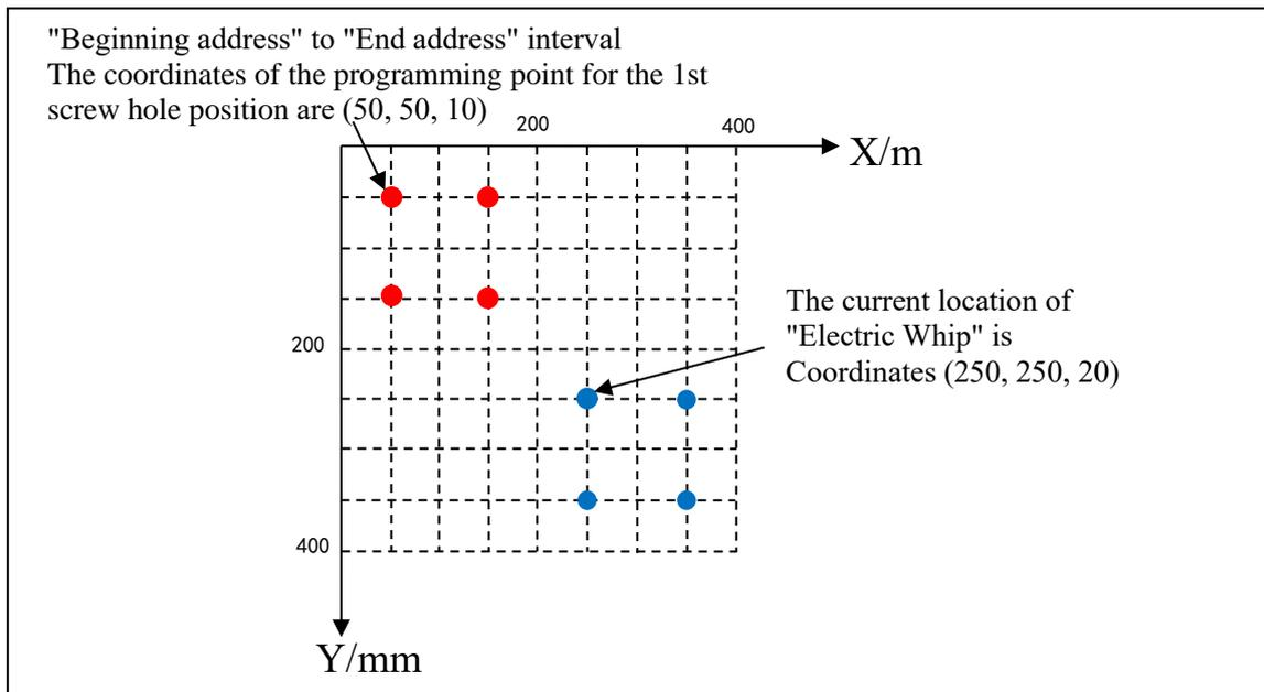
Figure 0.18 Schematic diagram of the "replication" principle corresponding to the case.
