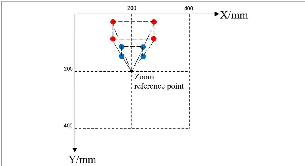
Figure 0.20 Schematic of "scaling" (a product reduced to 50% of its original
