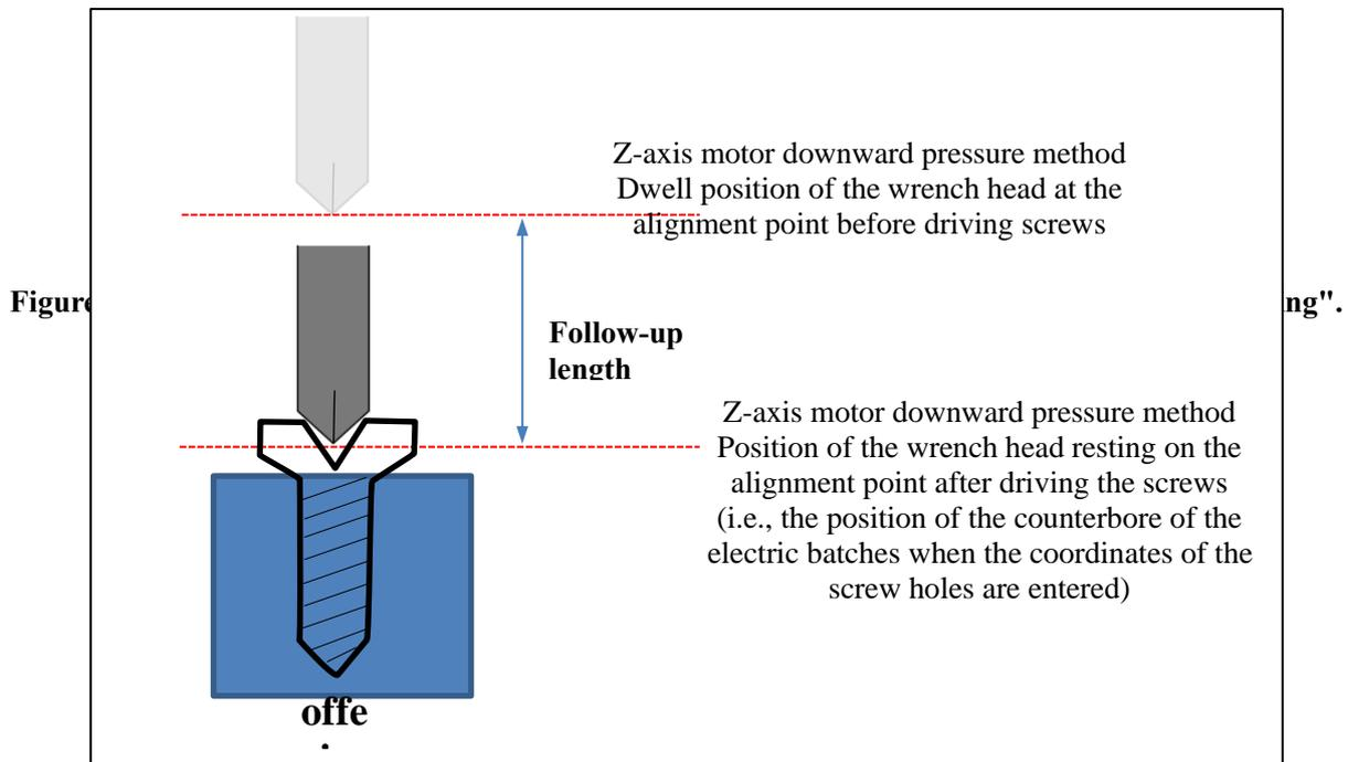
Figure 3.21 Schematic diagram of the "Z-axis motor downward pressure method" after
