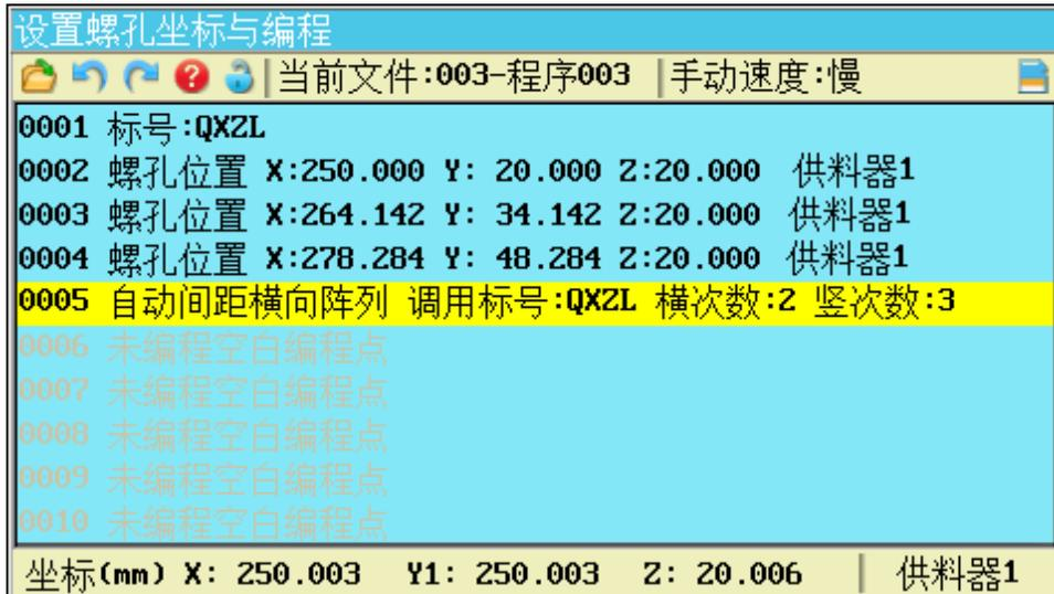
Figure 0 .28 Screenshot of the program for the case "Array with automatic calculation of spacing"
