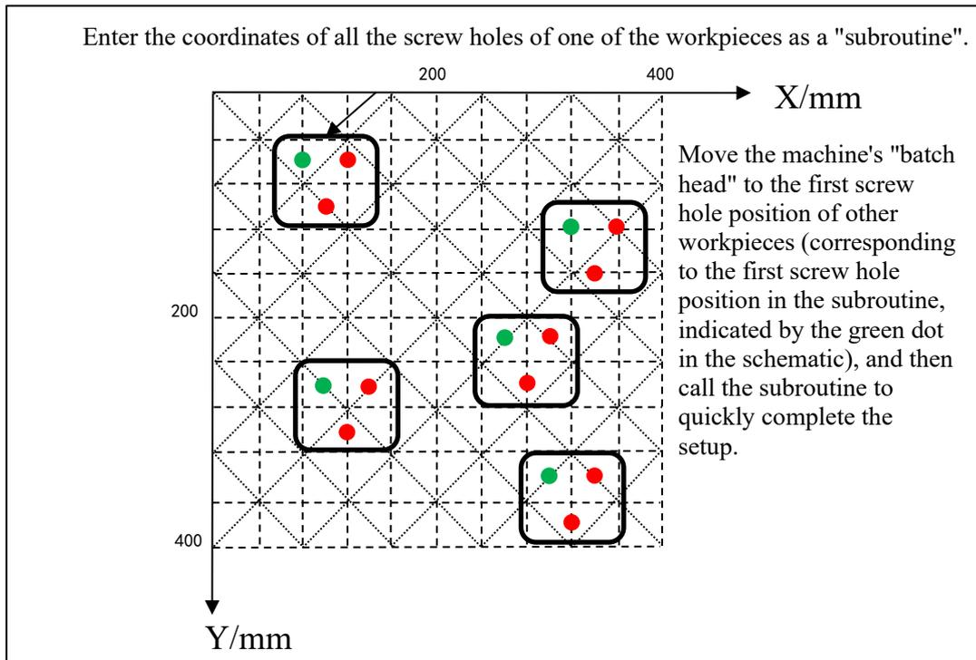
Figure 0 .34 Schematic diagram of the "calling subroutine" principle corresponding to the case.
