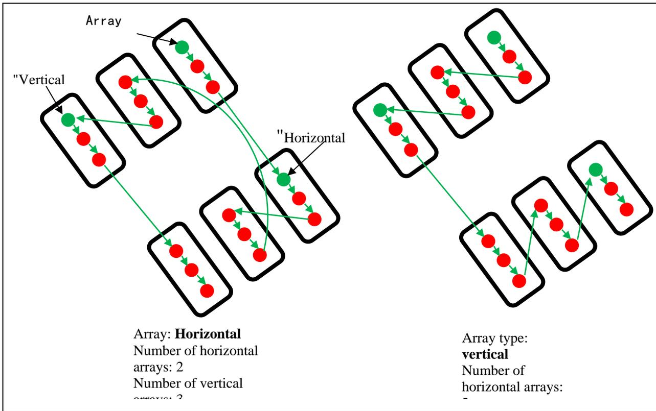
Figure 0.30 Top view of a workpiece with 3 screw holes arranged in the "Array with automatic spacing"
