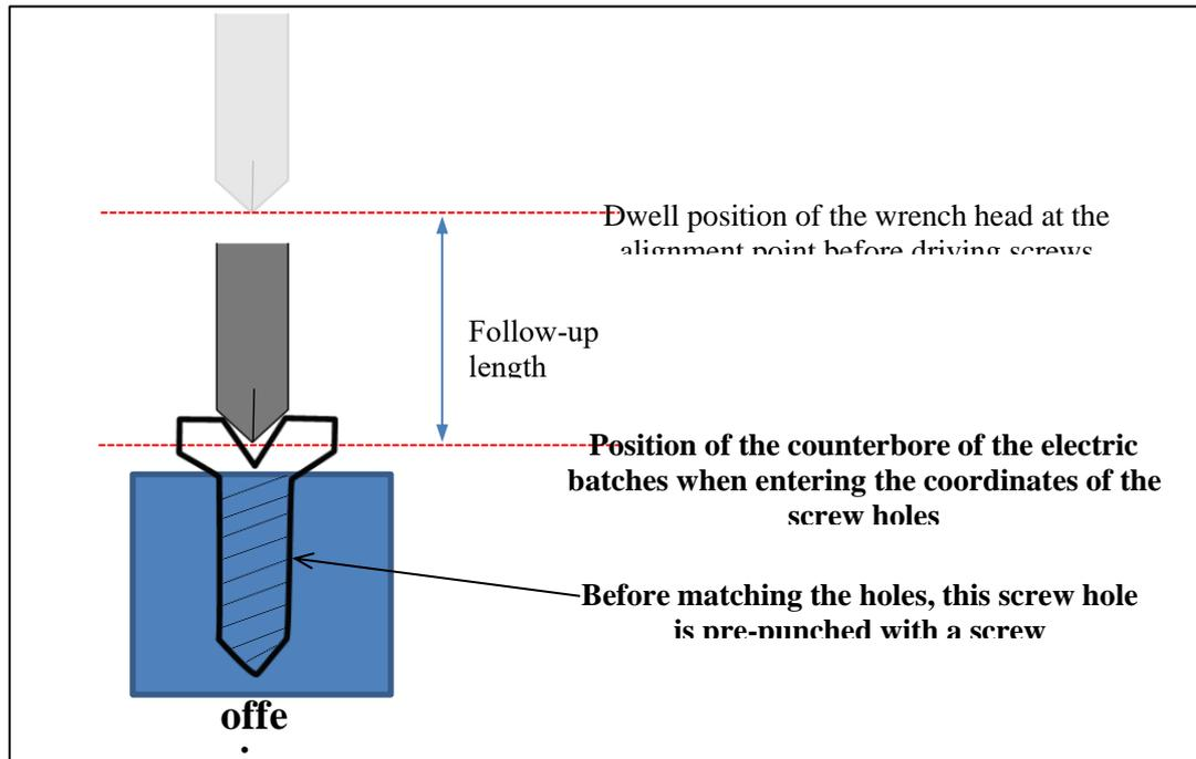
Figure 0 .14 Schematic diagram of the screwing method "Z-axis motor pressing down".
