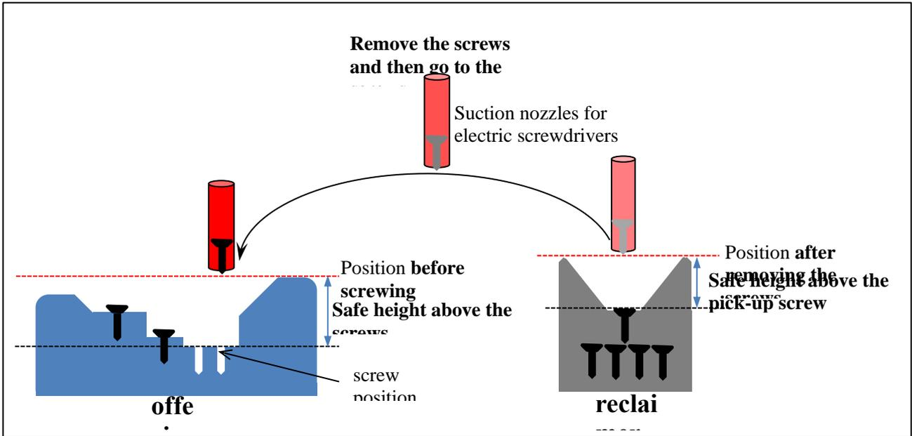
Figure 0.5 Schematic diagram of "Taking the screws and screwing them".
