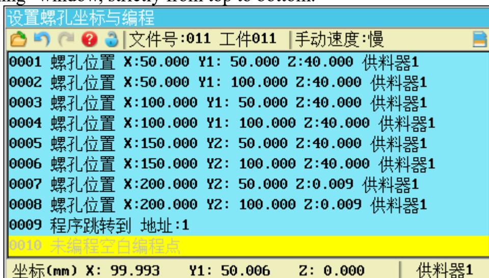
Figure 0.9 "Setting the screw hole coordinates and programming" window
