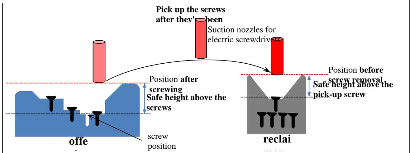
**Note:** ①The above schematic diagrams of "picking up the screws and then screwing" and "picking up the screws after screwing" are for the "suction" type of feeding machine. ②When using the "blowing" type material supply machine, you only need to configure the "safe height above the screw" parameter, even if you configure the "safe height above the screw" parameter, it will not be effective. Even if "Safe Height Above Screw Taking" is configured, it is not effective.
