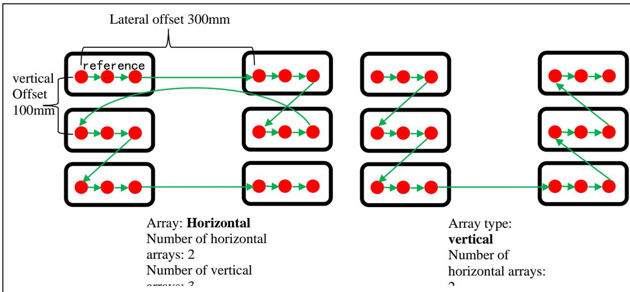
Figure 0.26 Top view of a workpiece with 3 screw holes arranged by the "Array with constant pitch input".
